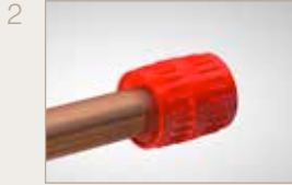
Deburr the tube internally and externally.
