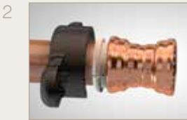
Clip the insert onto the tube and push the demounting tool into the clip. Continue to push to release the fitting.
